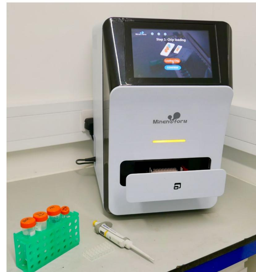
*MiNano-form: a high-throughput nanoparticle formulation system and the microfluidic cartridge developed at UCD.*
